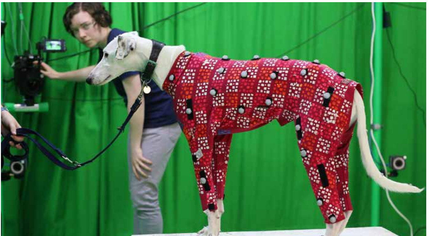
Sinead Kearney adjusts the cameras to collect the motion capture data of a lurcher. Photo credit: University of Bath
